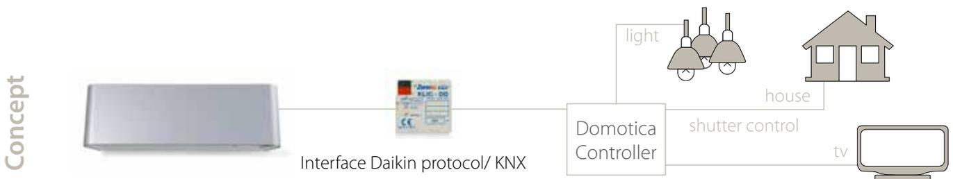
Connect Sky Air / VRV indoor units to KNX interface for BMS integration
