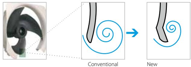
Escaping edges are sucked in by the bent blade edges, reducing overall turbulence.
