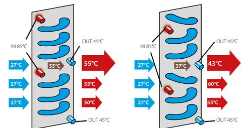
In cooling mode, the heat exchanger of the condensor is improved. This means an improvement of COP by 3%.
